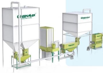
In 2022, the Company launched an EPS foam recycling and reuse system, a highly efficient device that integrates grinding, dust removal, dust collection, and mixing. The system grinds waste foam into pellets, removes dust to separate qualified materials, and mixes them with new materials to produce recycled panels, thereby achieving circular resource utilization.
